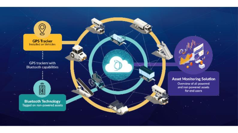
Our installation of GPS trackers with Bluetooth capabilities enables accurate location, movement, and condition monitoring of all air site vehicles. To track non-powered assets, Bluetooth sensors are tagged to them, which continuously broadcast signals. The GPS trackers, acting as gateways, pick up these signals, capturing all assets within proximity.
