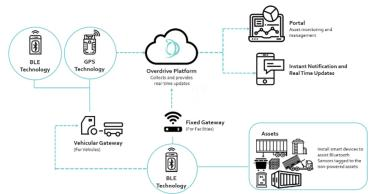
Bluetooth sensors tagged to the trailers (assets) were proven to be exceptional because of their practicality and ultra-low power qualities. Because of its low-powered nature, it enables the battery life to last up to 3 years without a charge. Thus, reducing the need for replacement and manual checkups.
