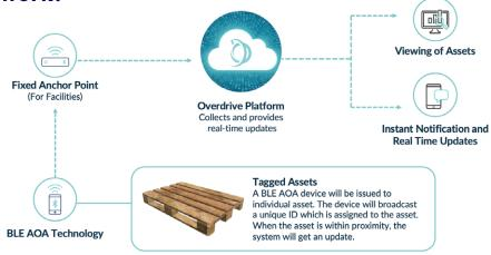
Bluetooth beacons are tagged in the pallets, containers and other individual assets which consistently broadcast signals. Fixed Anchors are placed in strategic locations to constantly listen to these signals.
