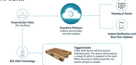
Bluetooth beacons are tagged in the pallets, containers and other individual assets which consistently broadcast signals. Fixed Anchors are placed in strategic locations to constantly listen to these signals.
