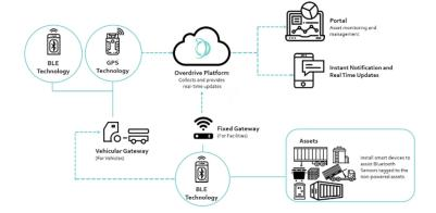
Bluetooth sensors tagged to the trailers (assets) were proven to be exceptional because of their practicality and ultra-low power qualities. Because of its low-powered nature, it enables the battery life to last up to 3 years without a charge. Thus, reducing the need for replacement and manual checkups.
